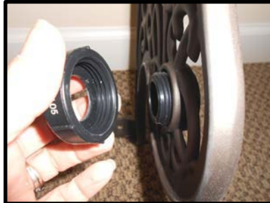
Hold the elbow stationary to unthread the swivel
