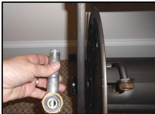
Hold the elbow stationary to unthread the swivel
