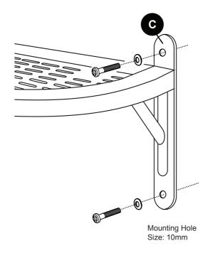
TIP: Remember to use the correct size and quantity of hardware to properly support the total weight of the unit. A standard 100' length of garden hose weighs approximately 15 lbs. Filled with water the additional weight can exceed 20 lbs. The mounting hardware must be able to support the combined weight of the unit, garden hose, plus water.
